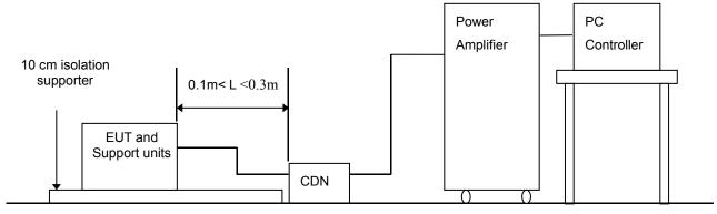
Note: 1. The EUT is setup 0.1m above Ground Reference Plane
